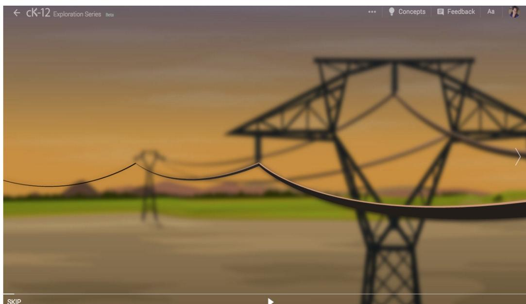
Power stations generate alternating current and voltage. Electrical transformers are used to increase the electric potential enormously (to hundreds of kilovolts). Power lines have small, but not zero, resistance, that depends on their material, diameter, and length. This nonzero resistance means that when the wires carry current, small voltage drops occur from one tower to the next. Is much electric power lost? Let's play around in the simulation.
