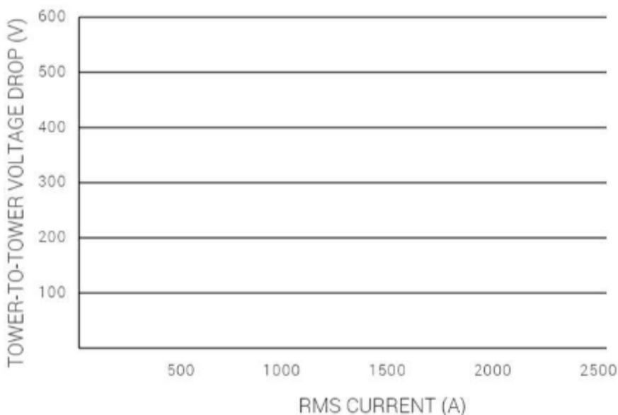
**Tower-to-Tower Voltage Drop Vs. RMS Current** - This is a plot of the RMS voltage drop (vertical axis) vs. the RMS current (horizontal axis) in the power line. The slope of this graph is a measure of the electrical resistance of the length of wire.
