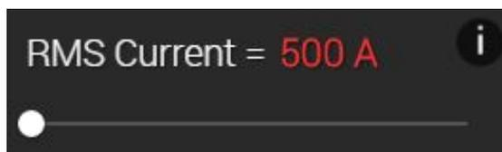
**RMS Current** - Since the current swings from positive to negative, through zero, its average is zero! The 'rms' (or root-mean-square) gives us a ballpark sense of the overall amount of current flowing one way or another at any given amount of time.
