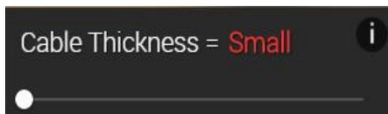
**Cable Thickness** - Thicker wires have more conducting paths through which the electrons can travel, and therefore have lower overall electrical resistance.
