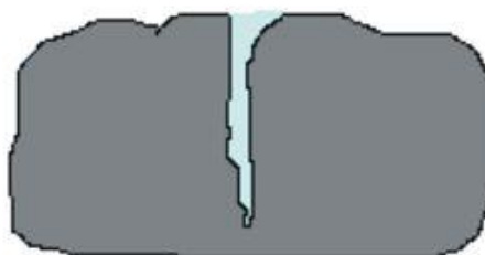
When the water freezes, it expands about 9% in volume, which wedges apart the rock.
